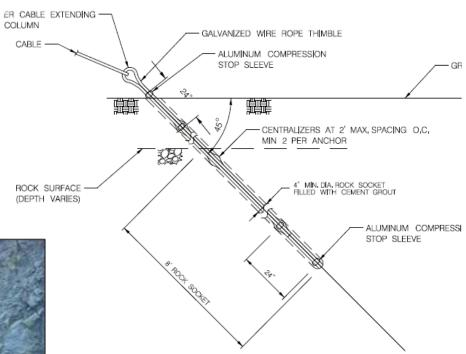
TYPICAL LATERAL WIRE ROPE ANCHOR P. N.T.S.
